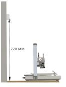
Drill two holes in the wall for the plugs, following these recommendations: Position the centers of the holes at 720 mm and 745 mm from the table surface for the lower and upper holes, respectively. These measurements ensure compatibility with the AMS lite cable length and proper spacing.
