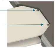
Remove the protective film from the Wall Mount Acrylic Sheets. Attach the Sheets to the AMS using the screws that came with your AMS. Use the M3 washers to protect the sheets. For additional stability, you can use two extra screws per sheet.
