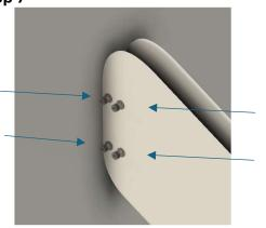
Attach the Wall Mount Arm Acrylic Sheets to the Wall Mount Block using 4x M4x10 Hex bolts and M4 washers on both sides.
